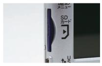
SD slot designed for easy checking of SD /SDHC card insertion
